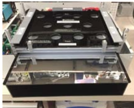
Insertion of Opaque Hand Enclosure into Optical Stack
