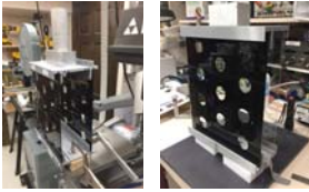
Optical Stack Assembly Solvent for Plastics: Methylene Dichloride
