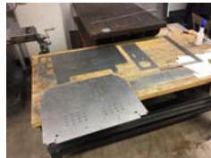
Parts Ready for Bending in a Brake
