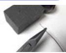
Wire held with welding pliers at the base of the twisted bare wire.
