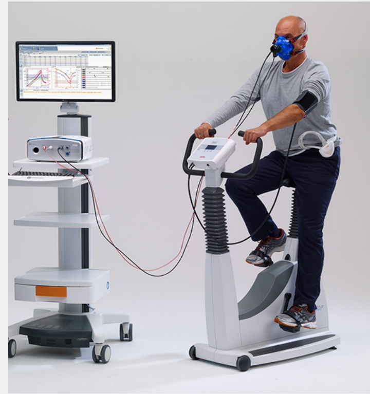
Vyntus® CPX Metabolic Cart and pedal ergometer, showing mask with gas sensors.
