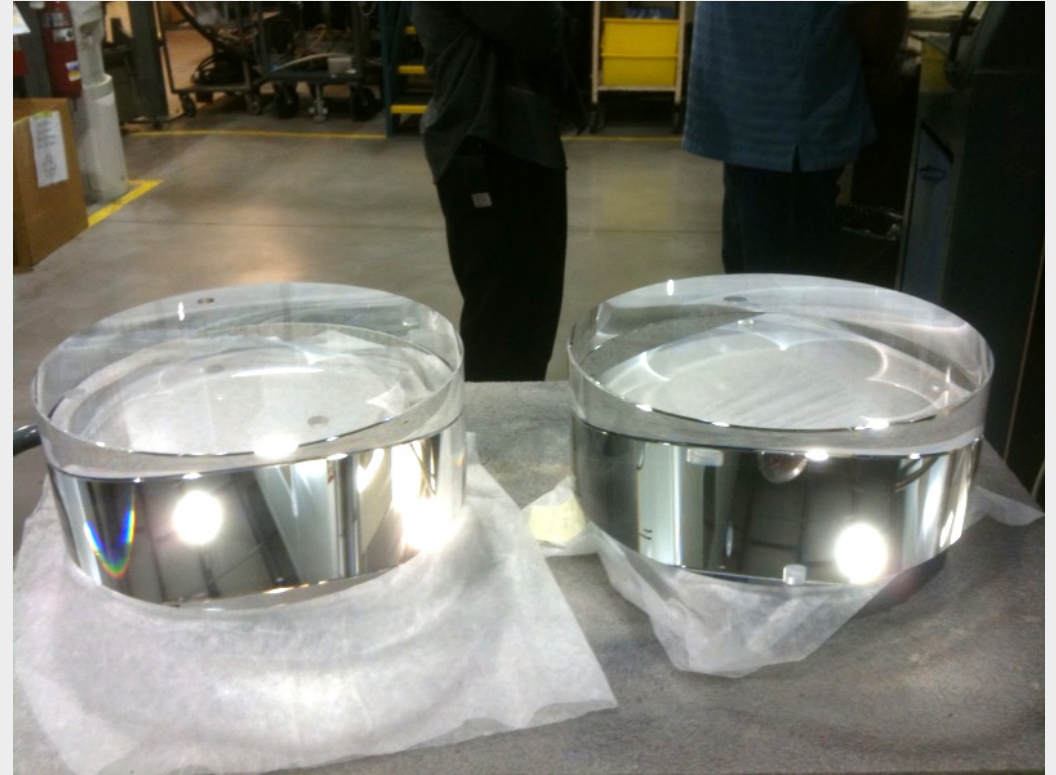
Two of LIGO's pure fused silica mirrors. 40 kg
