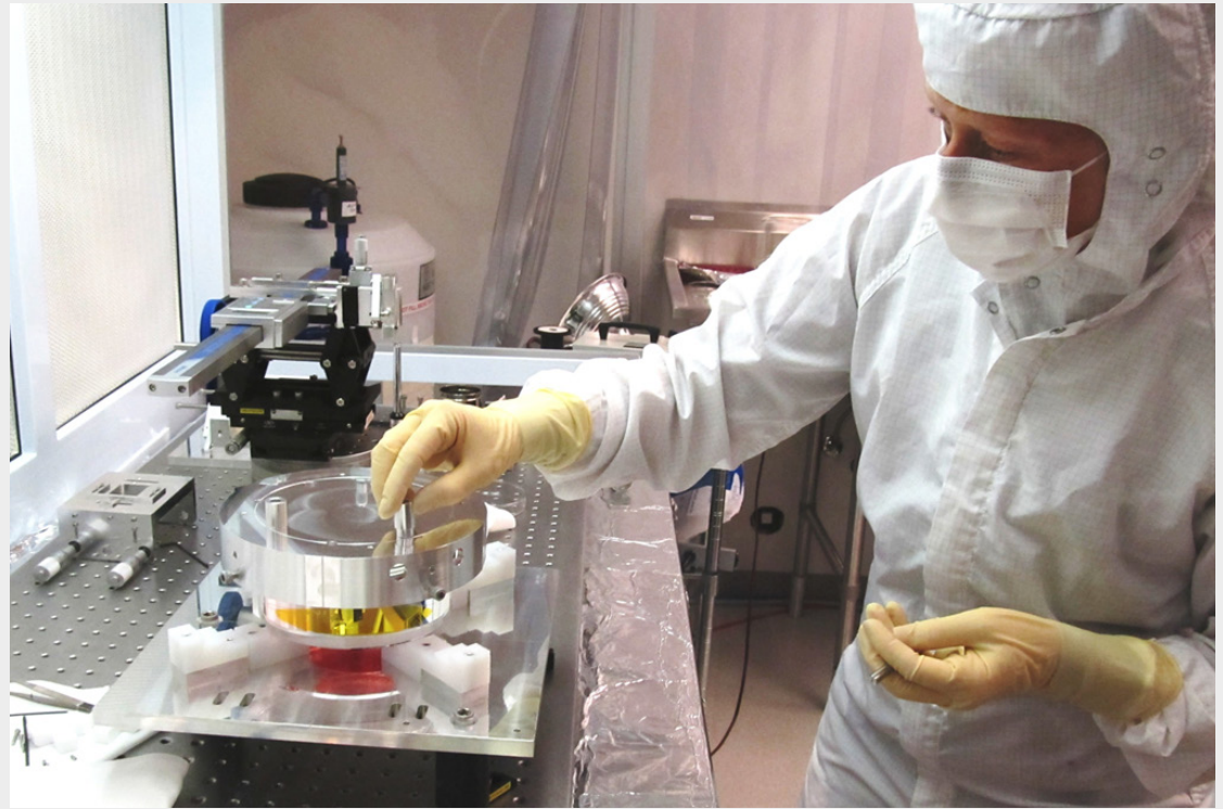
Preparing an optical mode cleaner for installation.
