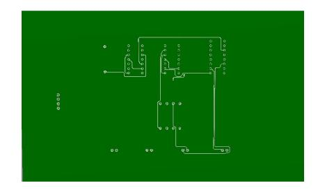
To have this board manufactured you must export the file with relevant information concerning the physical properties of the copper clad board, silk screen layer, and even the holes through the board (vias). The export dialog is as follows:
