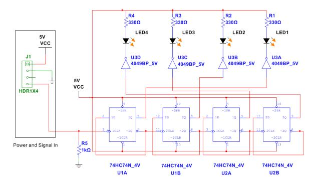
The resistors may initially have no manufacture's footprint for placement on a circuit board. Double clicking on the part opens its feature dialog. Under the "Value" tab at the bottom, "Edit footprint" is selected, and a suitable footprint chosen from the list available. If you were producing this board, you would want to be sure that each footprint matched the actual part you plan to use. Take a moment to inspect a part's features.
