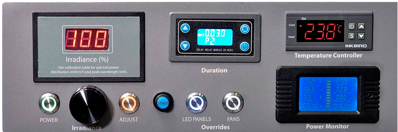
Fig. 3 The PTD console is located on the PTD’s right side and is not visible to a study participant. Irradiance (mW/m 2 ) and duration of exposure are set based on a study protocol. Irradiance (as a percent PWM) is determined in advance from the power level calibration
