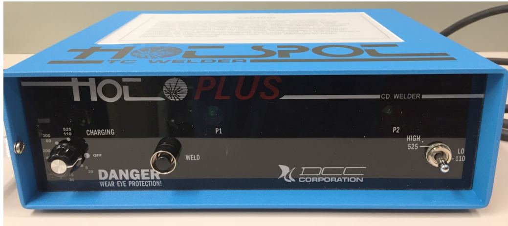
Front of the DCC Corporation Hot Spot Plus capacitive discharge welder. For more information see the appendix.
