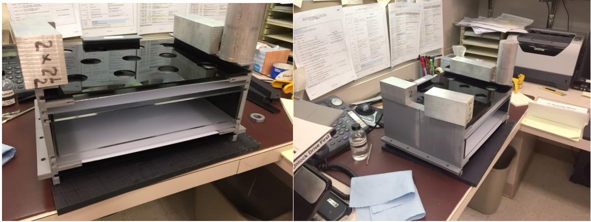
Solvent Bonding (Dichloromethane \text{CH}_2\text{Cl}_2 ) Optical Stack Parts in Prof. Saliterman's lab.
