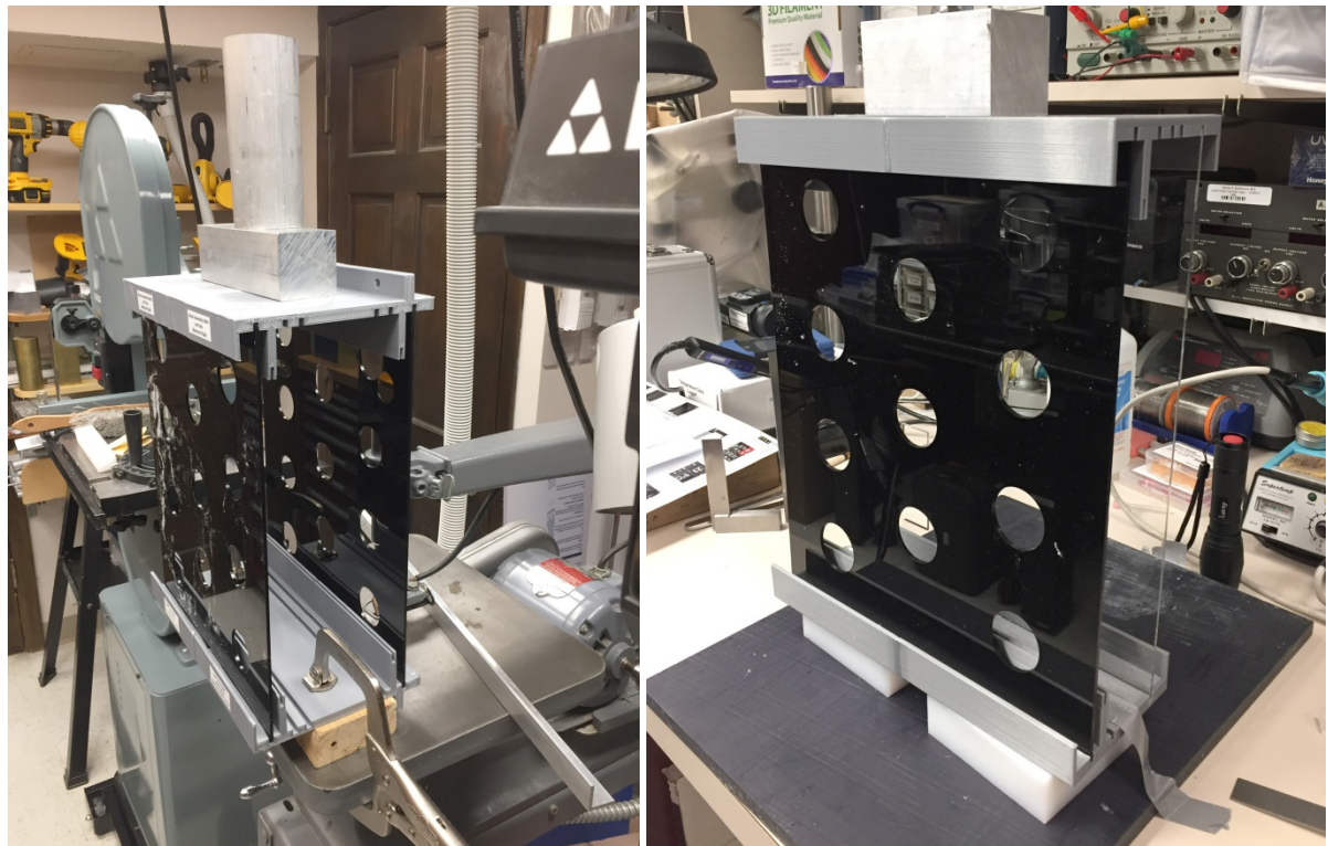
Solvent Bonding Optical Stack in Prof. Saliterman's lab
