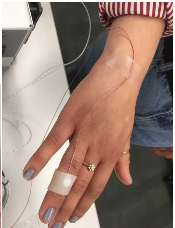
Test Placement & Fastening Technique for Skin/Finger Thermocouple outside Prof. Saliterman's office. Medical grade paper tape works well.
