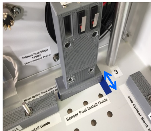
Sensor Post with microswitches - note positioning arrow.
