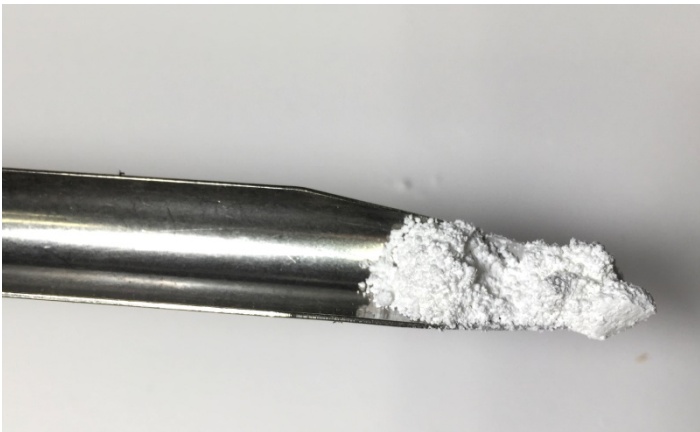
Add the Micro Lubrol (0.2g Hex Boron Nitride) Powder
