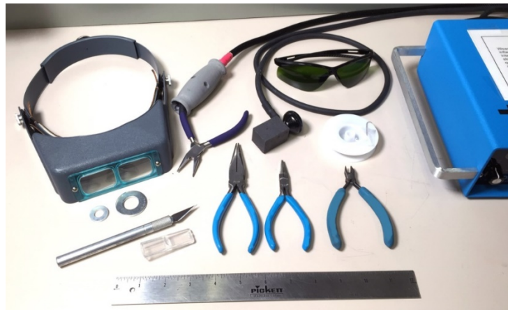
(Top Row) Magnifier, Welding Tool Holder & Mini-Pliers, Graphite Electrode Block & Cable, Thermocouple Safety Eyewear, Wire, Welder, (Bottom Row) Discharge Washers, X-Acto Knife & Cover, Long-Nose and Flat Pliers, Wire Cutter and Ruler.
