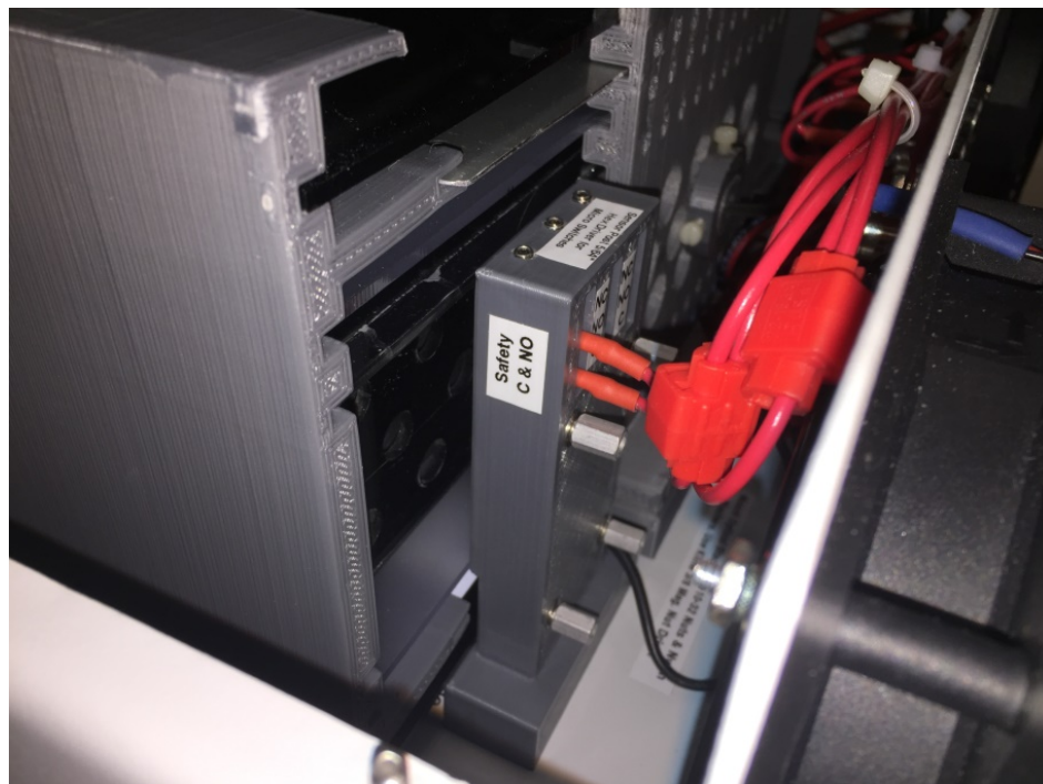
Correct Position of the Sensor Post
