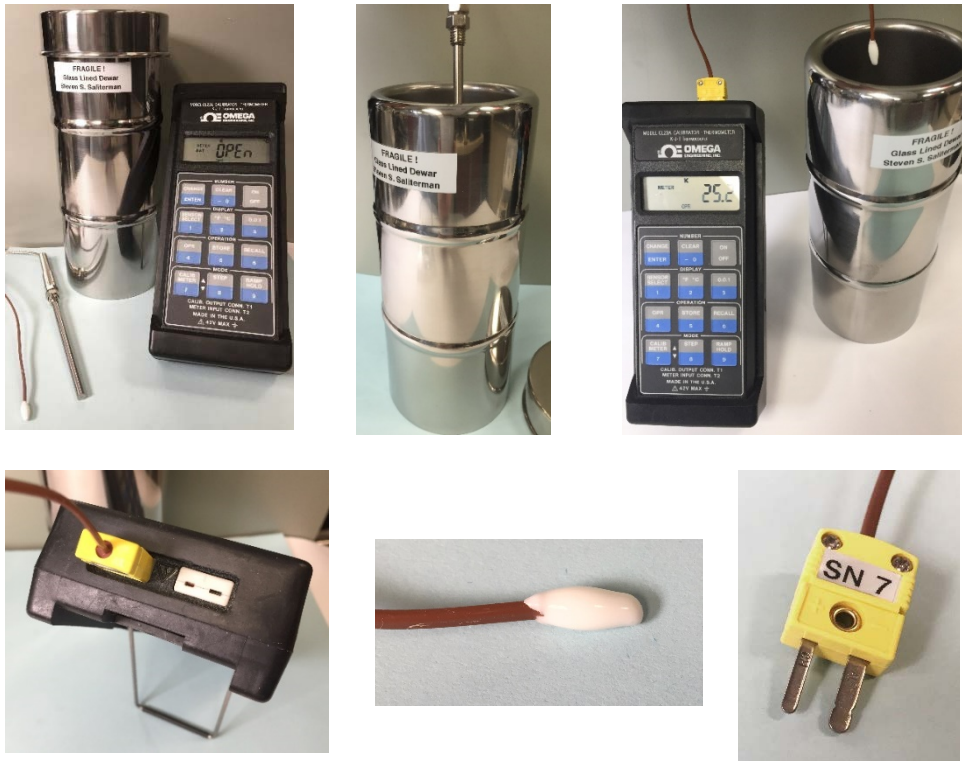
Thermocouple under test, reference TC, Dewar with distilled water ice bath, and the Omega CL23A Calibrator – Thermometer.
