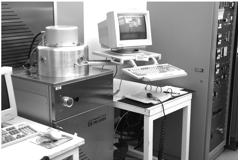
Figure 2.39 Plasma-enhanced chemical-vapor deposition station.
