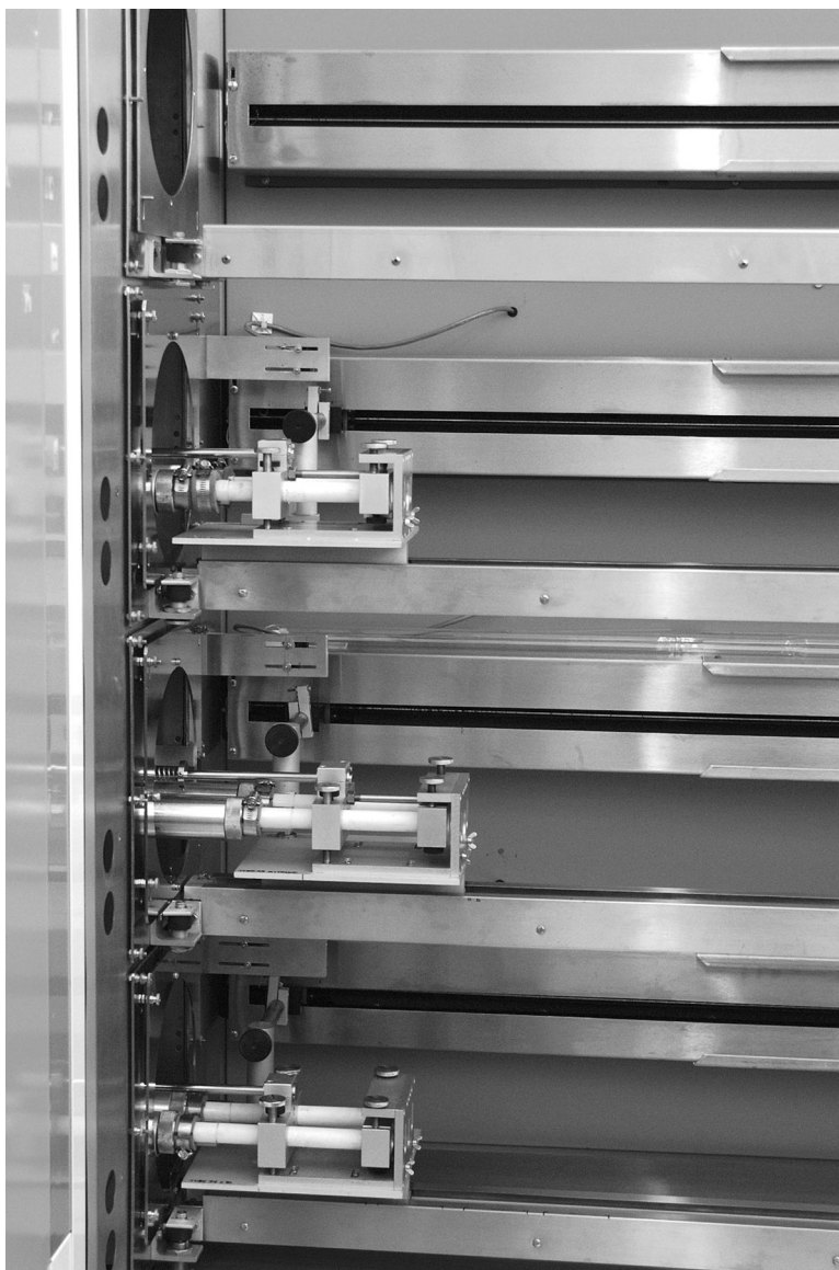
Figure 2.42 Loading chamber for the LPCVD system.
