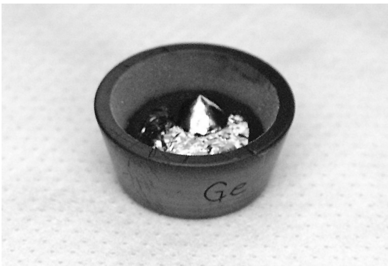
Figure 2.34 Graphite crucible filled with germanium for evaporation.
