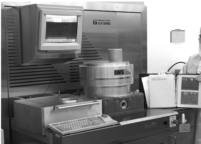
Figure 2.52 Deep reactive ion etching (DRIE) machine.
