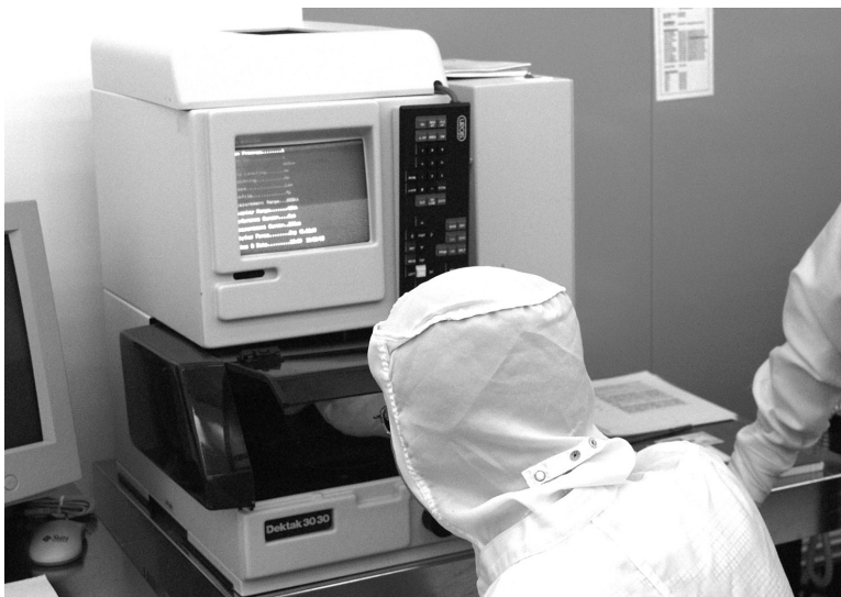
Figure 2.27 Profilometer for measuring surface features, including depth and width of etched structures.
