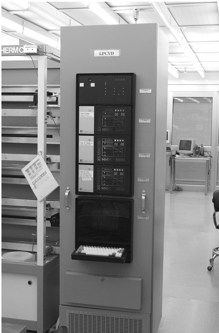
Figure 2.41 Low-pressure chemical-vapor deposition system (LPCVD).
