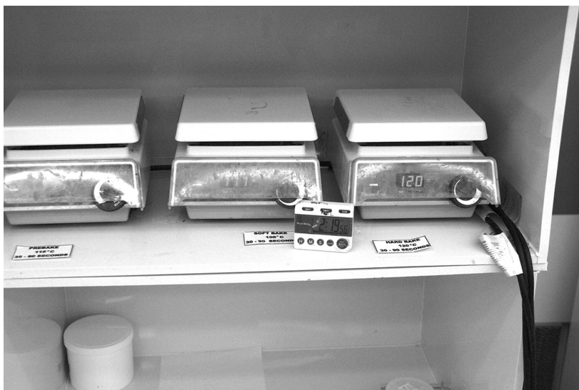
Figure 2.14 Silicon wafer soft and hard baking plates.
