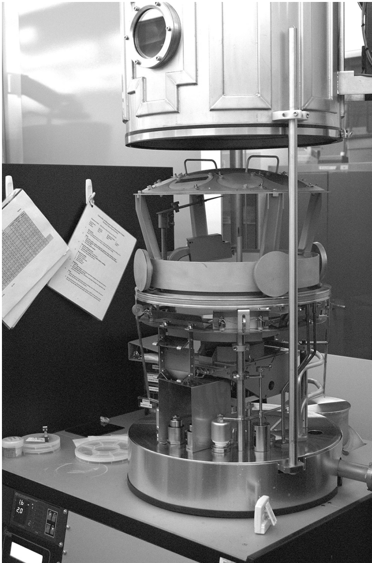
Figure 2.32 Electron beam machine (open for setup).
