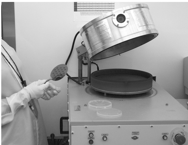
Figure 2.24 Placement of the silicon wafer into the RF RIE machine.
