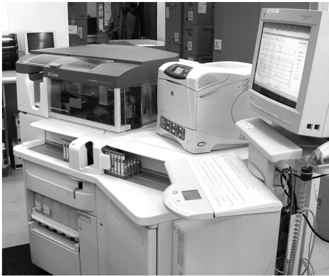
Figure 8.4 This system uses chemiluminescence to tag antibodies, replacing traditional radioimmunoassays. Tests include thyroid (TSH, free T4), tumor markers (CA-125, CEA) and hormones (testosterone, estrogen).
