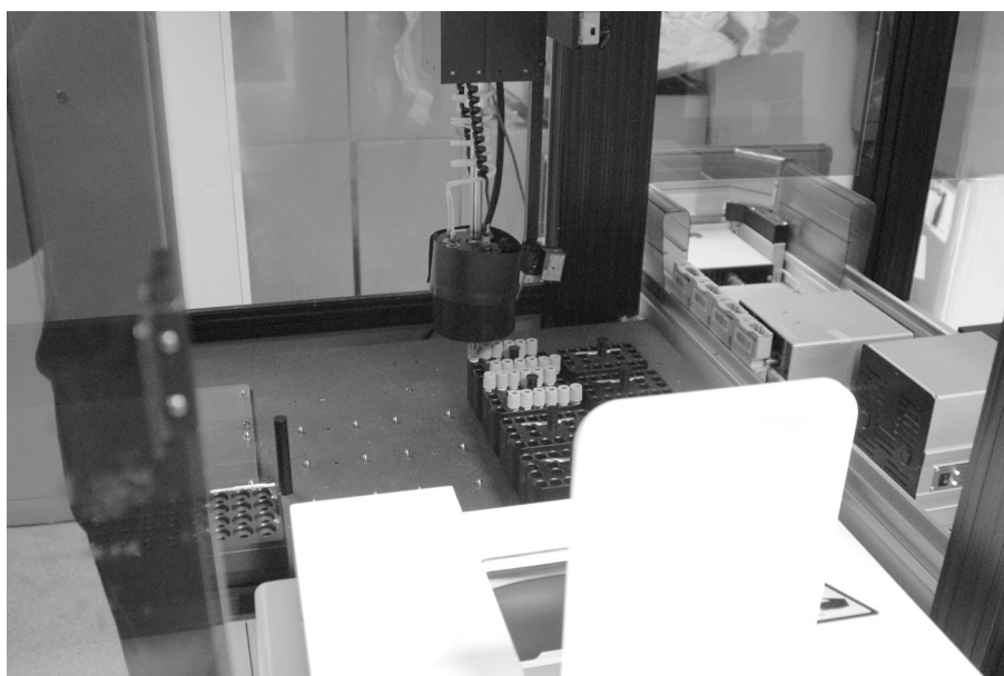
Figure 8.2 Close up of the LAB Interlink system with centrifuge (in the foreground) and robotic manipulator arm.
