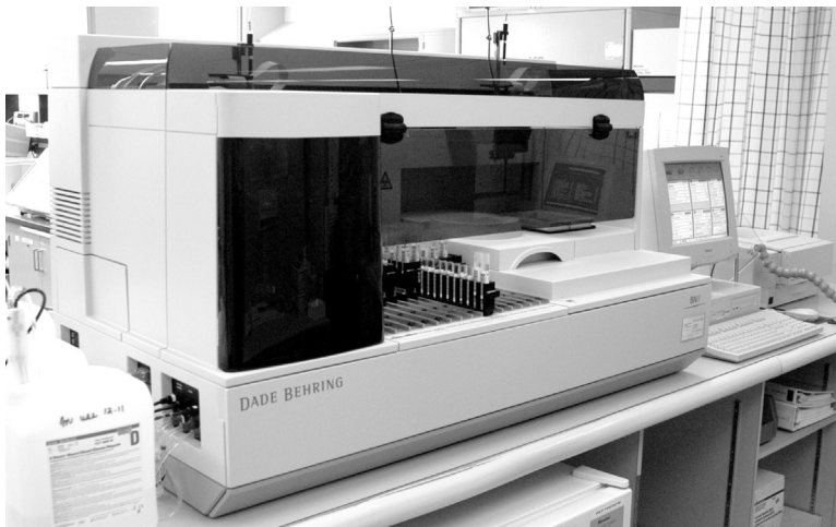
Figure 8.6 The nephelometer is capable of performing IgG, IgM, rheumatoid factor, transferrin, prealbumin and haptoglobin studies.
