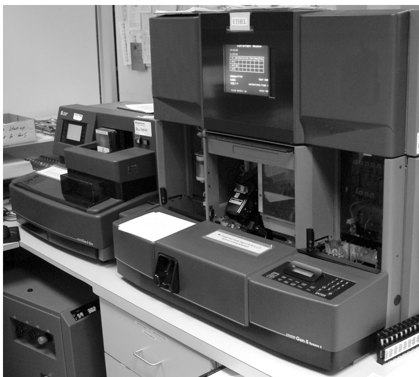
Figure 8.8 The Coulter Counter GEN S performs complete blood counts (CBC). This includes a built-in slide maker and ability to perform reticulocyte counts.
