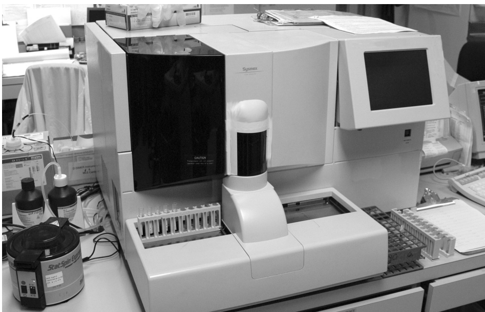
Figure 8.15 The Dade Behring coagulation analyzer is able to detect clot formation for protime (INR) and partial thromboplastin time (PTT).
