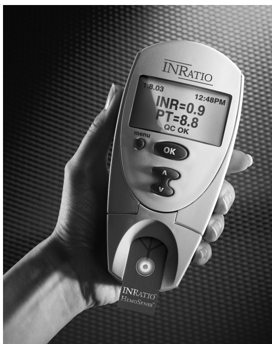
Figure 8.16 The HemoSense INRatio Meter shown is a hand-held device for point-of-care use. (Photo courtesy of Hemosense, Inc.)
