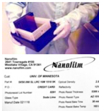
Unexposed Masks (Resist is Pre-applied)
