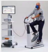
Vytus® CPX Metabolic Cart and pedal ergometer, showing mask with gas sensors.
