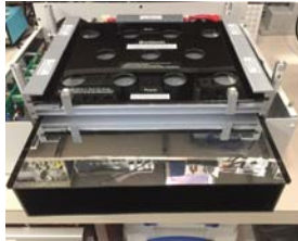
Testing Insertion of Opaque Hand Enclosure into Optical Stack
