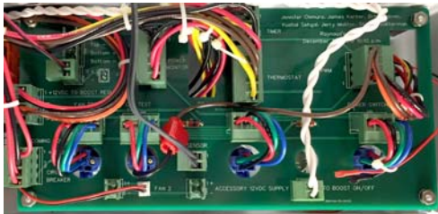
Printed Circuit Board – Primary Junction Point for Switches, Meters, LED Panels, Power Supply and Fuses
