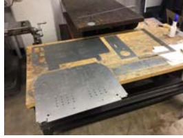
Parts Ready for Bending
