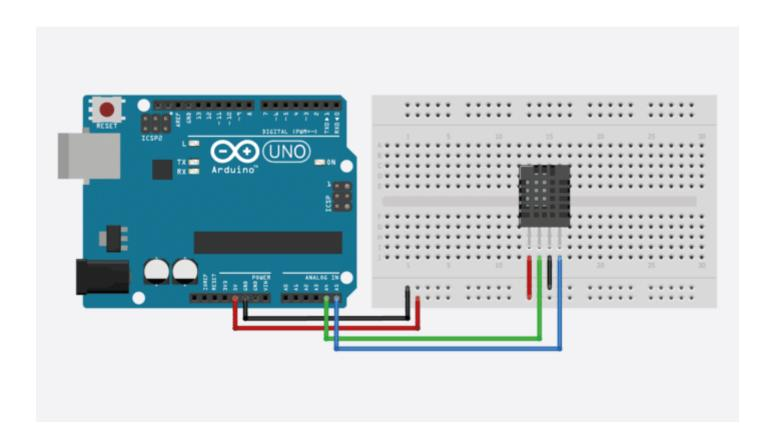
In this tutorial, you will learn how to use the AM2320 digital temperature and humidity sensor (https://amzn.to/35P5DsU) with Arduino. I have included a wiring diagram and example code to help you get started!
