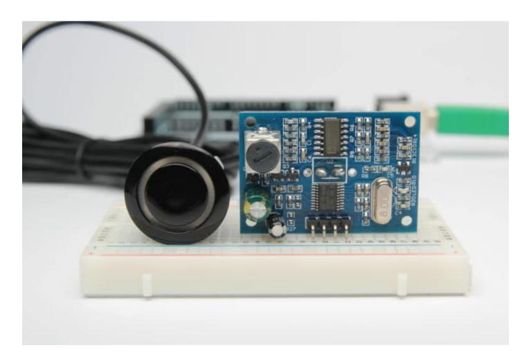
The JSN-SR04T (https://amzn.to/2XdsHeH) is an easy to use waterproof ultrasonic distance sensor with a range of 25 to 450 cm. If you are planning to build a water level measuring system or if you need to take other distance measurements outside, then this is the sensor you need!
