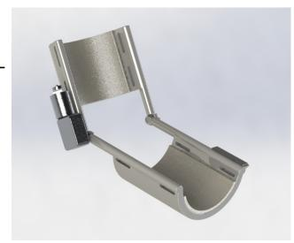
tiometer to one half of the joint and then fixing the cap of the potentiometer to the other half of the joint. This signal would then be sent to an Arduino that would convert the changing resistance to an angular displacement. It would then display your progress and your improvement based on previous data. In addition to a system which can calculate an angle based on the resistance from a potentiometer, the team also included a timer with which users could set their therapy time.
