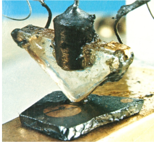
Point-contact transistor 1947, Bell Labs (Brattain and Bardeen).
