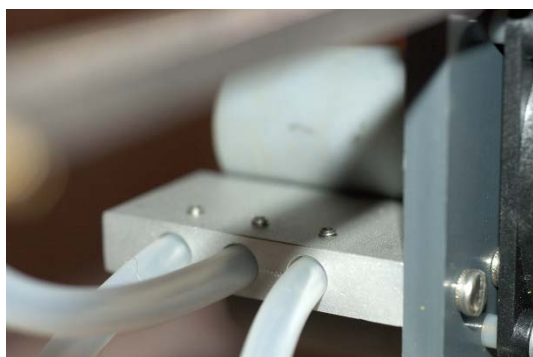
Catheter Guideway to Optical Encoder
