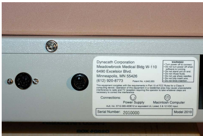
Rear Power and Computer Connectors, Labeling
