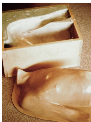
Torso Mold and Fiberglass Casting
