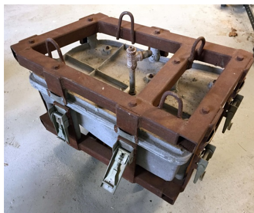
Assembled Mold for Rotational Molding
