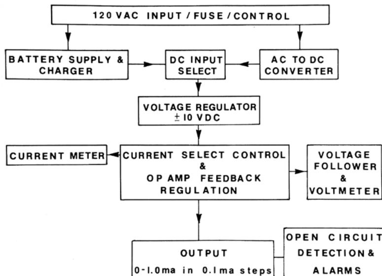
**Fig. 2** Front panel and block diagram of the stimulator. Current is set between 0 and 1.0 mA with the current step switch. The current meter reads the current selected in mA, and the voltmeter reads the voltage. The O.C. (open circuit) light and audible alarm warns of an open circuit or defective electrode.
