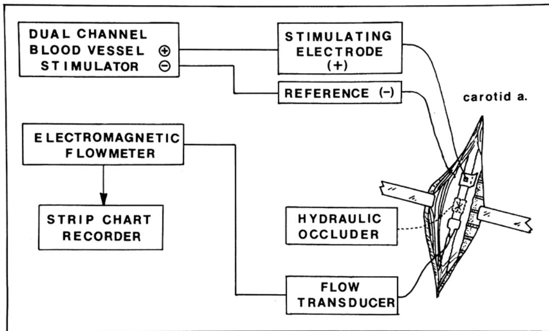
**Fig. 3** Arrangement of the instrumentation during the acute study. Current levels of 0.5 and 0.7 mA were chosen for the study. The flowmeter (Zepada Instruments, SWF 4-RD) was connected to the flow transducer only when the stimulator leads were disconnected. The recorder displayed phasic and mean flow. The stimulator reference electrode was sewn into the adjacent muscle. During the chronic study, a miniature hydraulic occluder was placed between the transducer and stimulating electrode.
