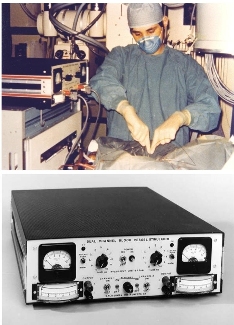
**Fig. 9 Top**, Attachment of stimulating electrode and flow probe. **Bottom**, Constant-current power supply.
