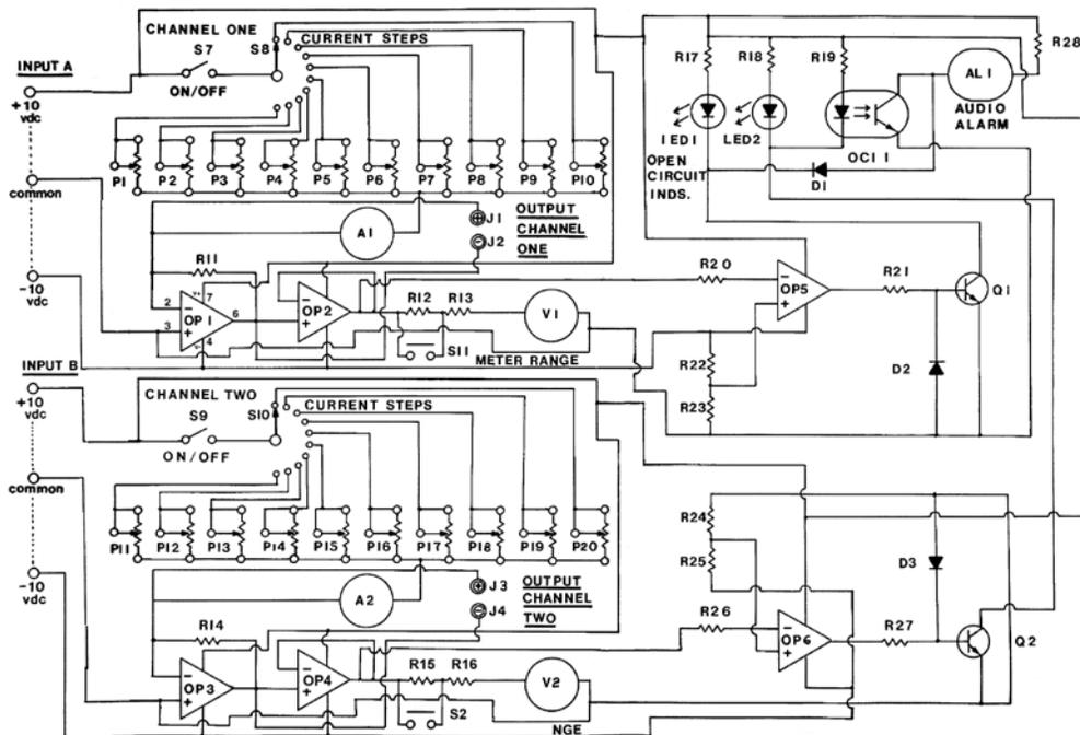
**Fig. 11 Top,** Charger and regulated DC input circuits. **Bottom,** Current selection, high-impedance operational amplifier feedback drive circuits, and alarm circuits<sup>18</sup>.
