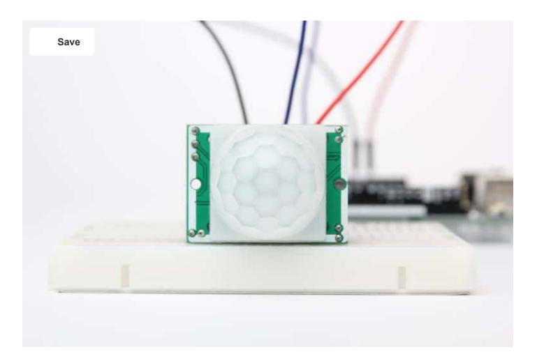
In this tutorial, you will learn how the HC-SR501 PIR motion sensor works and how you can use it with Arduino. You can find Passive Infrared (PIR) sensors all around you, they are not only used for security purposes, but also in most automatically-activated lighting systems.
