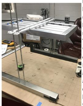
health care providers commonly switch between conventional (3 bulb) and intensive (5 bulb) levels of phototherapy by removing the individual bulbs. This commonly causes damage to the bulbs by dropping them or breaking the lamp holders. In order to fix this issue, we added a switch to the device and changed the circuitry in order to be able to easily change between conventional and intensive phototherapy.
