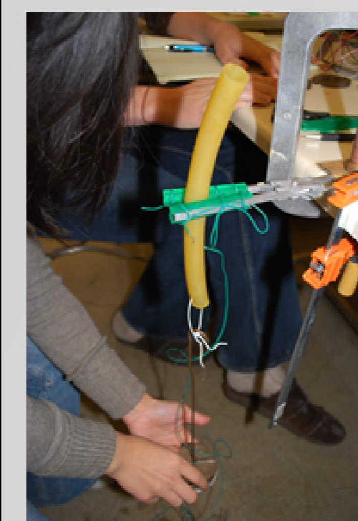
Figure 8: Experimental setup of slipping test, tubing is used to model the aorta.
