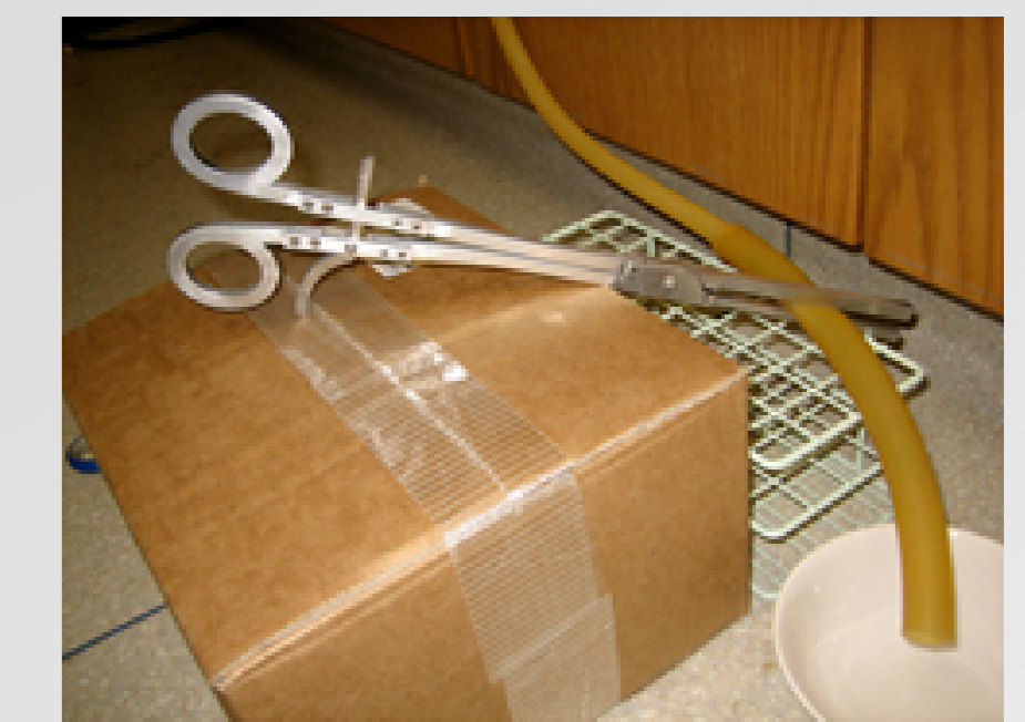
Figure 11: Setup for testing the clamp's ability to occlude flow for six hours under physiological blood pressure.
