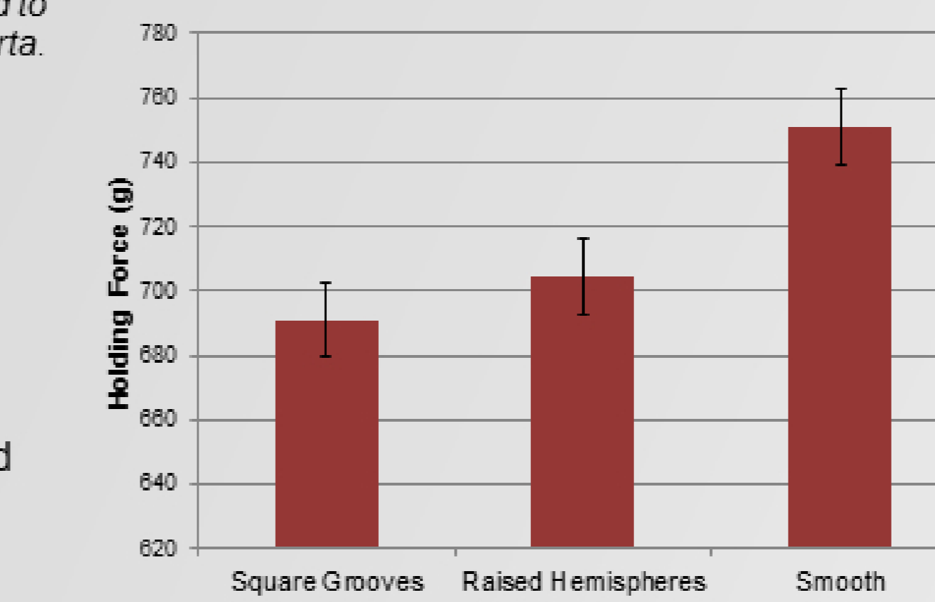
Figure 9: Holding force for various jaw insert surface characteristics
