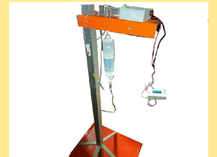
Automated Infusion Monitoring System
