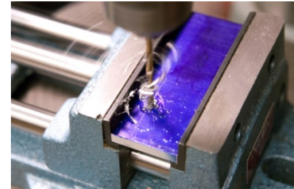
Drill - take short pecks - lifting drill every so often to release chips.
