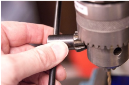
Replace spotting drill with #29 drill bit. Remove the key!
