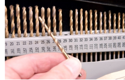
Select the #29 drill for an 8-32 tap (per the chart).
