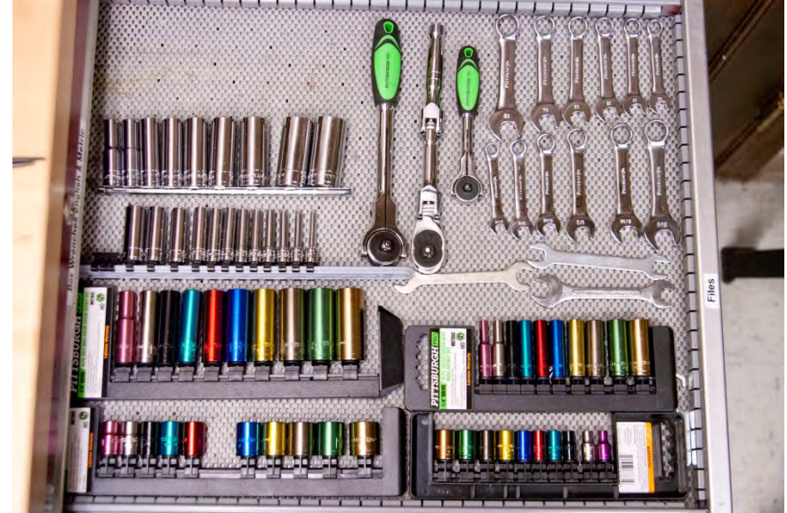
English and metric, standard and deep socket wrenches; handles and stub box wrenches.
