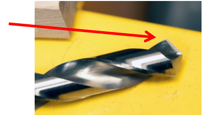
Drill bits for Plexiglas and polycarbonate.
