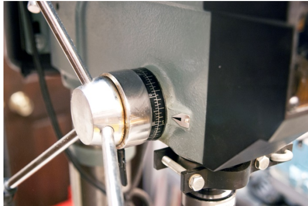
Hand feed and depth adjustment.
