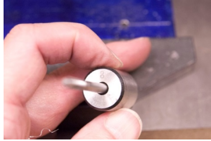
Place and tighten into #8 adaptor.
