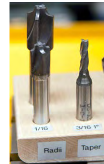
Corner Rounding (Radius) & Taper
