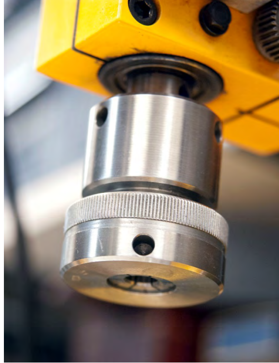
Spindle, collet holder & collet.
