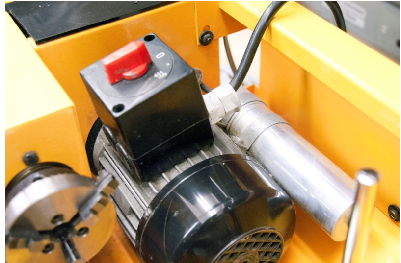
Motor and motor capacitor.
