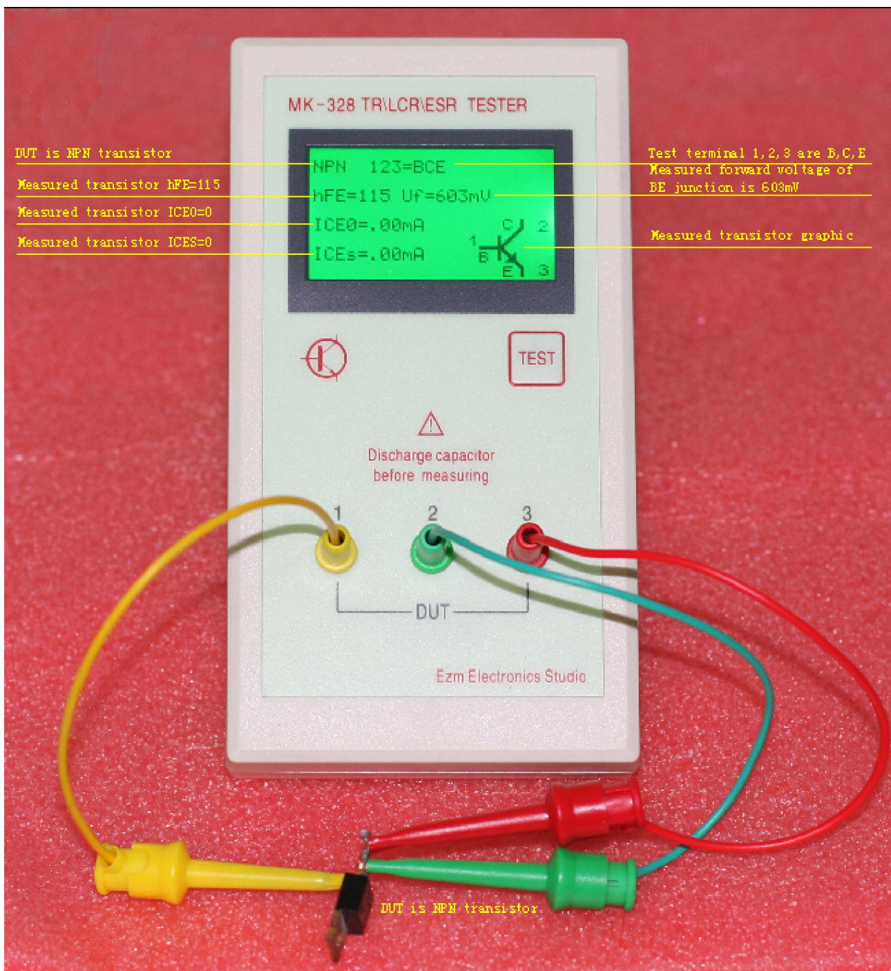
Figure 4: Test Transistor with Test Clips
