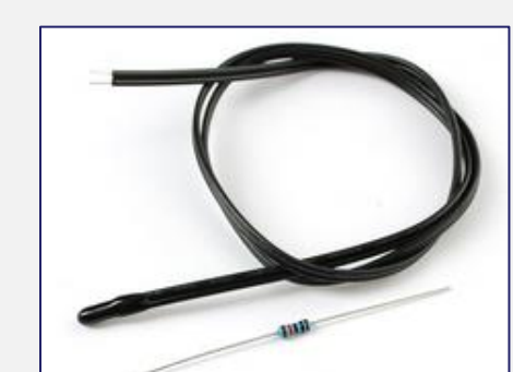
Figure 4: 10K Precision Epoxy Thermistor used in SensIschemia Retractor.
