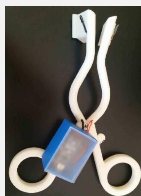
Figure 6: Final prototype, with wires running from the sensors to the box containing the Arduino and battery.
