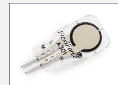
Figure 3: FlexiForce A301 sensor used in SensIschemia Retractor.
