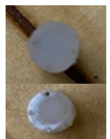
Figure 3: Images of silicone molds following laser cut step. A) Although the small holes are difficult to see, this piece was cleanly cut and able to be removed and overall shows promise for this methodology. B) This piece shows more damage caused by the laser, possibly suggesting the settings should be reassessed. However, it was still easily removed and the holes are present.
